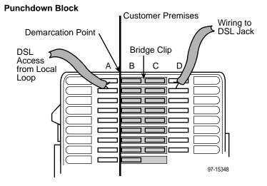
3. Locate the DSL pair of T1/R1 connectors on the customer premises side of the NID or punchdown block. Attach the wiring that will be connected to the DSL jack. In the following example, a NID is used without a POTS splitter. It includes an existing POTS line and a second pair installed for DSL access.
